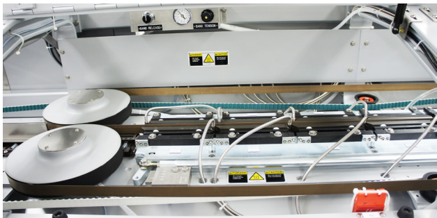
Heat seal section of the S-CH-S with (4) sets of heat bars.
